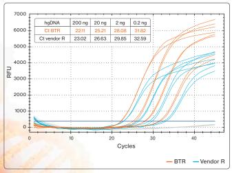
Superior results with high-sensitivity qPCR amplification. Human genomic DNA was diluted (200 ng to 0.2 ng per reaction) and amplified using ApStarTaq DNA Polymerase and an aptamer *Taq* polymerase from Vendor R to evaluate sensitivity and specificity. Results demonstrate distinctly earlier Ct values and higher signal of detection for the biotechrabbit polymerase.
