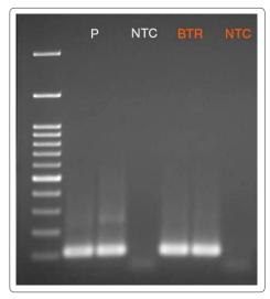
High-yield amplification. cDNA was synthesized from 500 ng human total RNA in a 50 µl reaction at 50 °C and subjected to 40 cycles of amplification of a 111 bp product using the One Step RT-PCR Mix and a kit from Vendor P. The biotechrabbit mix produced high yields and exhibited no amplification of side products, illustrating its high specificity. NTC: no template control.
