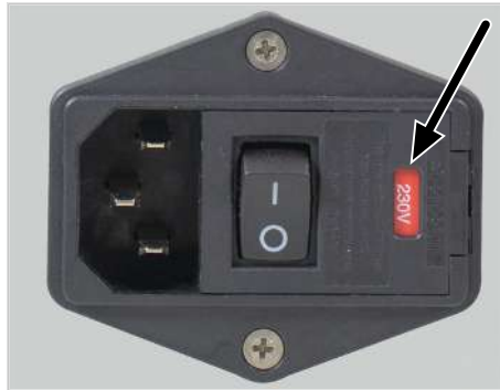
Fig. 9 Mains connection and fuse holder
