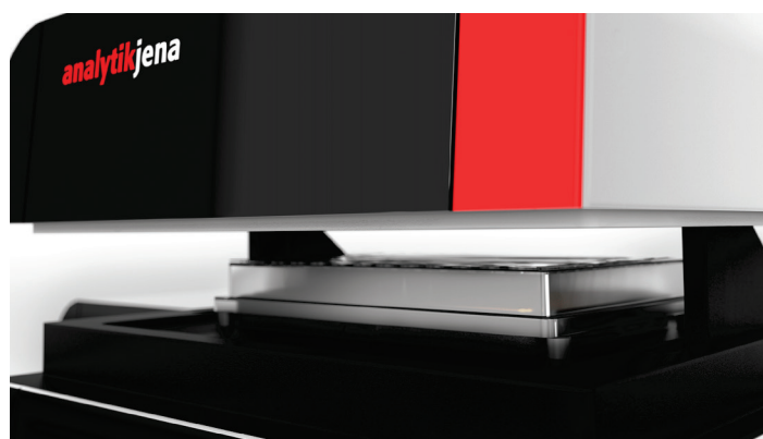
Fig. 4 Extended lifting pins lifting the sample plate with the lid already slightly open
