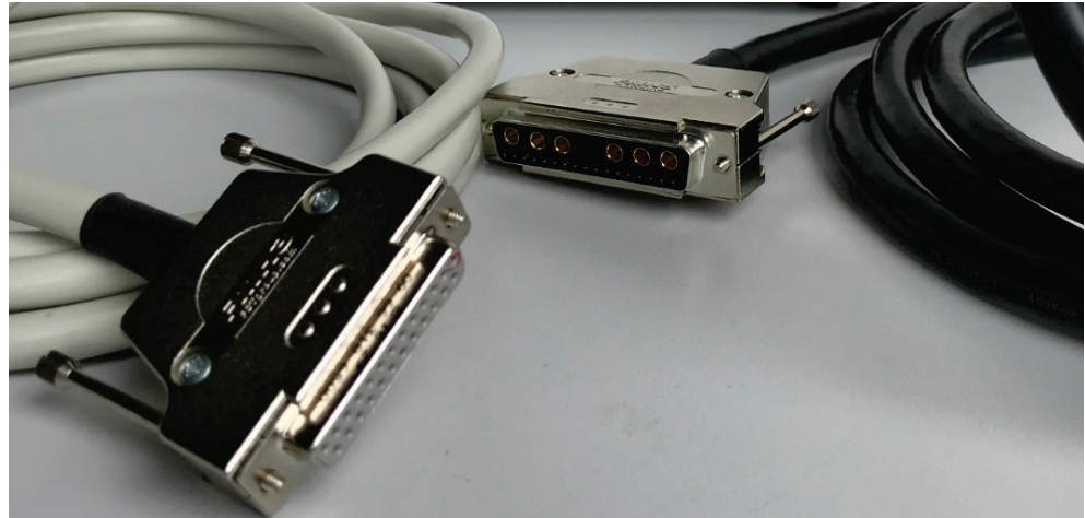
Fig. 7 Cables and connectors for connecting the PCR module to the controller. Left: DSub 24W7 signal cable, right: DSub 12 supply cable (cable colors may vary)
